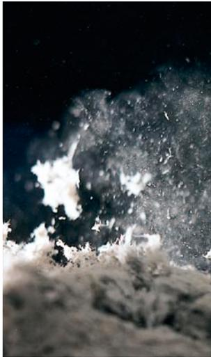
**Figure 1.1** Asbestos fibres being released from lagging
